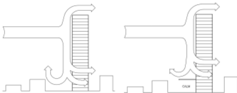
Figure 11: Canopy Windbreak Treatment. (L) Downwash to street level may generate windy conditions for pedestrians. This is particularly true for buildings much taller than the surrounding buildings. (R) A large canopy is a common solution to this pedestrian-wind problem at street level.
